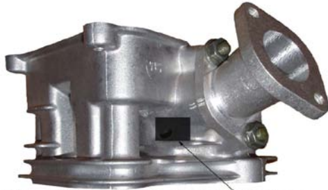
Approved Yamaha YF200 Inlet Tract Repair Area
